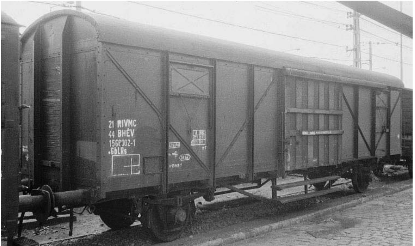
21 44 BHÉV 1568002-1 •GbLRs , with air brake Hik-GP. Peterszebet 25.06.1990 © Per Topp Nielsen Markings say load limit 20,0 t and floor 28,5 m 2 . Both are wrong - should be 22,0 t resp. 30,0 m 2 .
